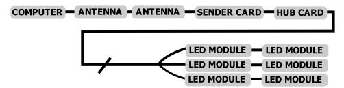
Some signs, especially if they are double-faced, will have one sender card and a receiver and hub card in each face. To view test patterns you must disconnect the connection to the sender card and then push the test button on the receiver card.
