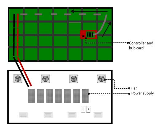
The data from the controller moves out through the hub card, and horizontally along each ribbon cable.
